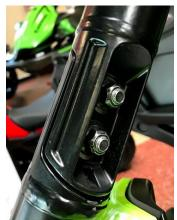
2. Locate the new A-Pillar brackets, bolts, spacers, washers, and nuts. The driver side assembly is shown below. Use the picture for reference to identify the driver side bracket. If the cage shifted after step one, it may be necessary to push the cage inward to realign the mounting holes.
