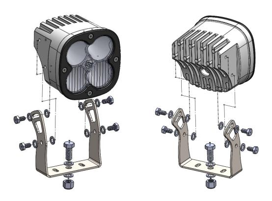
6. Mount lights onto the A-pillar brackets with the 3/8" hardware. After, Aim and tighten the lights using the 7/16" socket, 9/16" wrench, and 9/16" socket.
