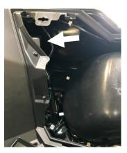
2. Remove the in-cabin rear access panel by pulling the top edge toward the front of the vehicle (see image on next page). The picture on the right below shows where the A-pillar light switch leads can be routed. The switch can be removed to route wires through and then reattached. Take note of switch terminal configurations.
